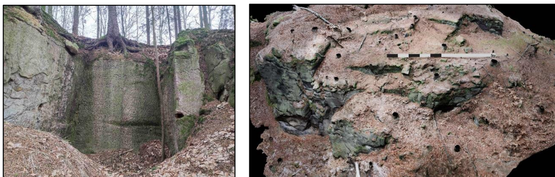
Fig. 2. Left: A deep incision with vertical walls, formed by sandstone wedging and detachment to produce building stone. The faces bear traces of chiselling (Pekelský důl Valley, carving with the year 1809) (photo Z. Vařilová). Right: a 3D model of the Dachslöcher Quarry, where strata-parallel, bench-by-bench extraction was conducted for the production of 185 pieces of masonry stones and 78 pieces of tiles (one-off mining in 1852 - State Archive in Litoměřice) (model by. J Horák).
