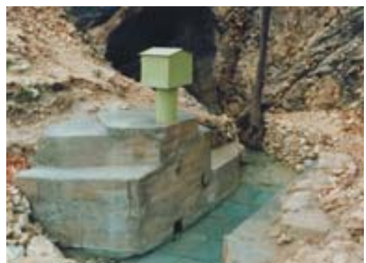
Fig. 5 - Karst spring with laminograph in Zagross basin
