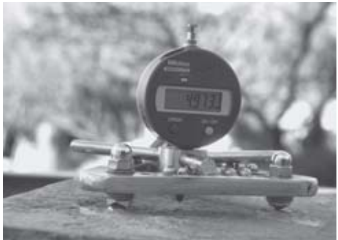
Fig. 2. The traversing micro erosion meter (TMEM)
